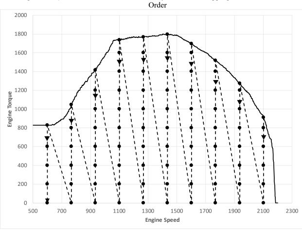
Figure 1 of § 1036.535—Illustration of Steady-State Fuel-Mapping Test Points and Run Order
