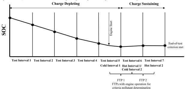
Figure 1 of § 1036.510—FTP charge-depleting criteria pollutant test sequence.
