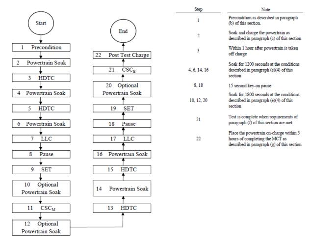
(f) The test is complete when the following end-of-test criteria during CSC<sub>E</sub> have been met.
