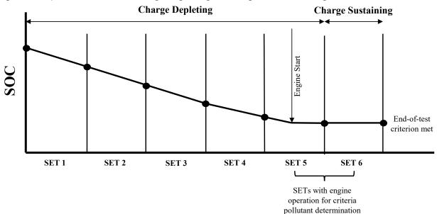
Figure 1 of § 1036.505—SET charge-depleting criteria pollutant test sequence.
